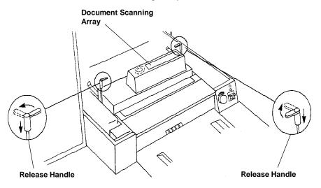
4. Push down and rotate the release handles outward to release the DSA assembly.
